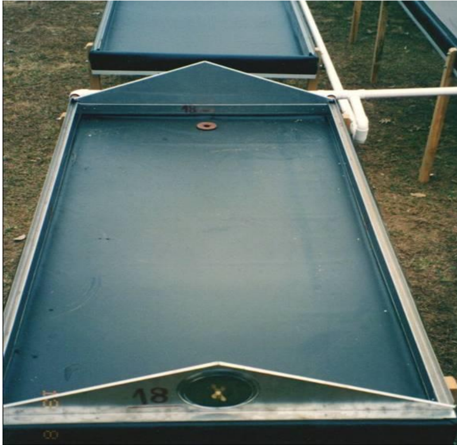
Figure 1.5: Solar Distiller used for removal of Arsenic from water by distillation.
