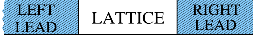
Figure 3.8. Geometry used for the calculation of the conductance. The interacting region (lattice) is connected by ideal contacts to semi-infinite ideal leads.
