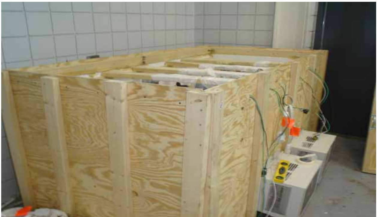
Figure 3-1: Climatic Chamber With Four Air Conditioners and Ten High-Powered Lamps.
