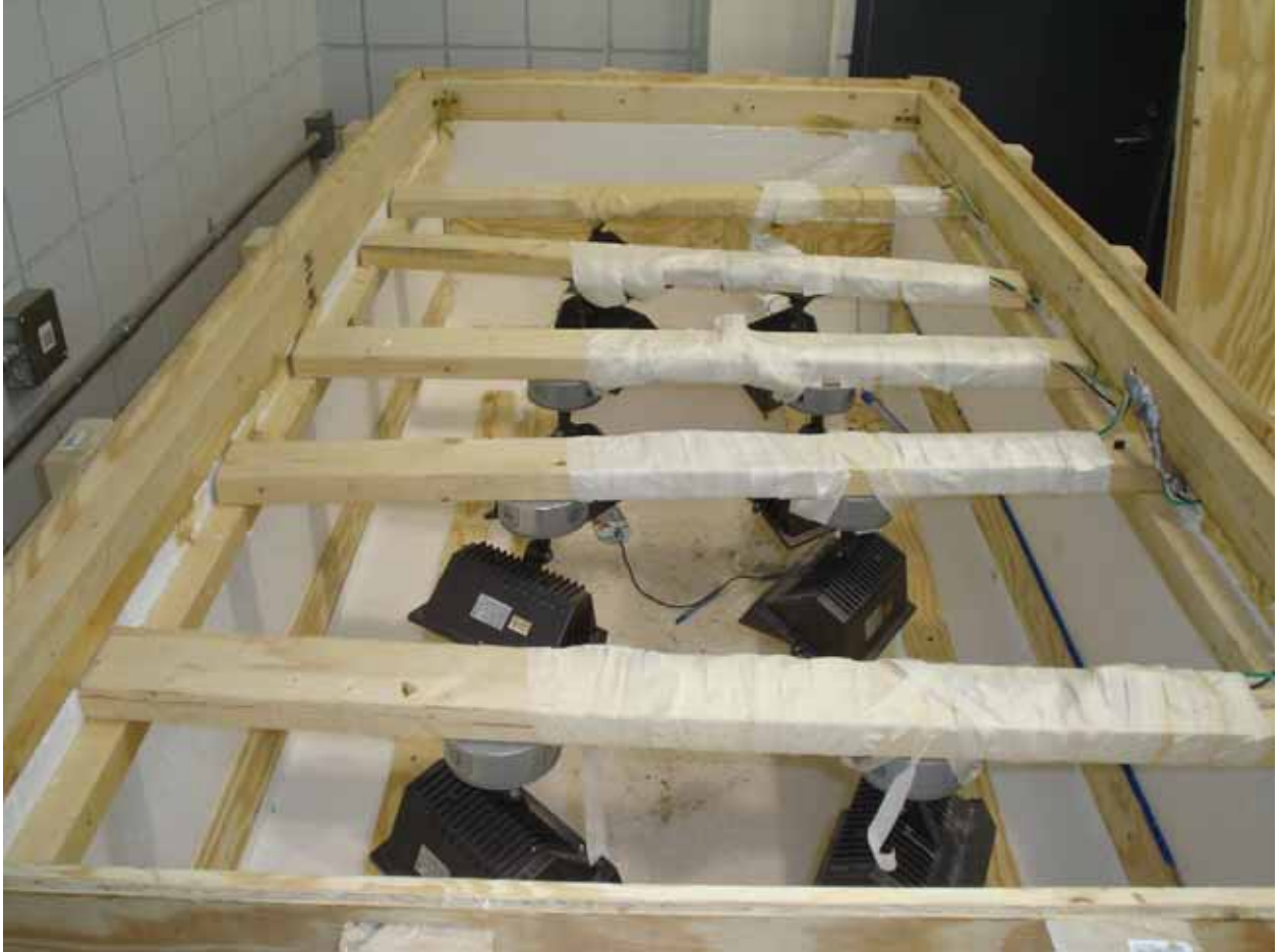
Figure 3-2: Plan View of Constructed Climatic Chamber and High-Powered Lamps.
