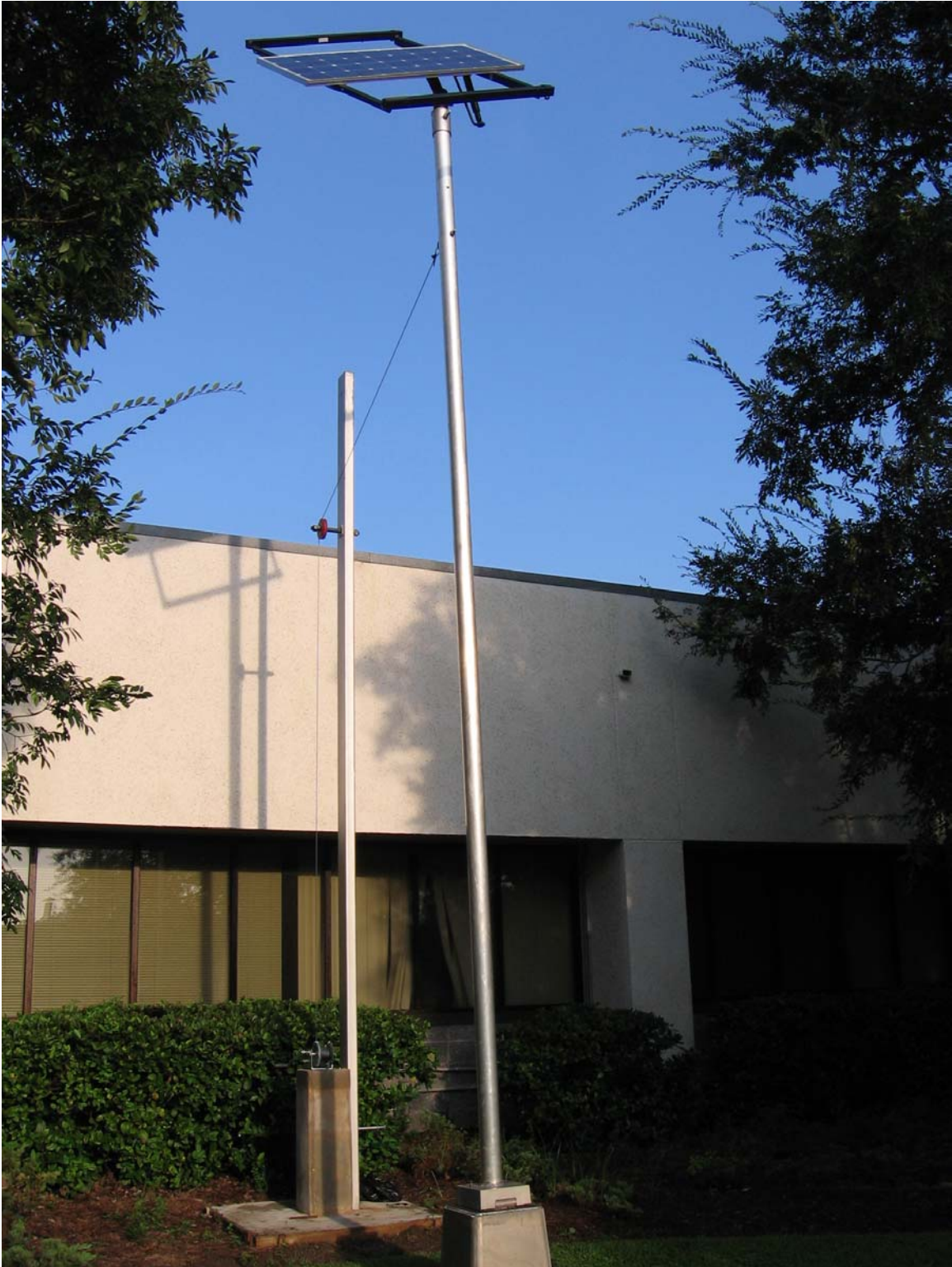
Figure 3.2 Photo of Completely Assembled Tracking System for the Research located at the Centennial building Innovation Park, Tallahassee.
