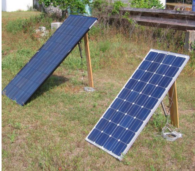
Figure 4.1c Data Collection Inclined at an Angle of Forty Degrees.
