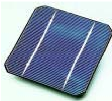
Figure 1.1 Photovoltaic Cell, the smallest device capable of converting sunlight to direct current electricity.
